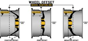
Purchase only high quality, properly sized, "HUB-CENTRIC" wheel spacers from reputable suppliers that match the MINI and Wheel hub size Always purchase longer wheel bolts (stock length + spacer thicknes) with the spacers. Check wheel bolt torque after installation and after driving a minimum of 100 miles multiple times until the torque stabilizes. The recommended wheel torque is 100 lb-ft [135 Nm]. www.ecstuning.com is a good source for high quality spacers and long wheel bolts.
