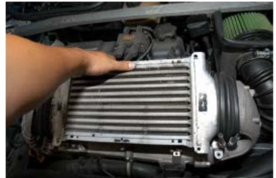
6. Remove the stock black rubber bellows and discard. These will be replaced with the new M7 silicone boots.
