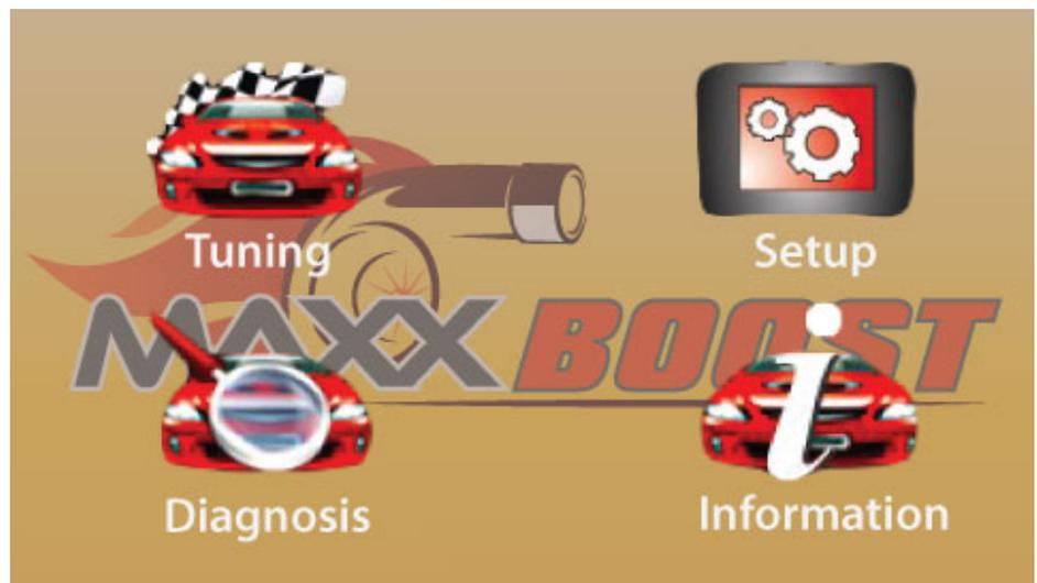
**Information:** To display the info about your MAXXBoost device (for ex. Serial Number, Hardware and Software version) and, in case you've already read a vehicle, the info about the ECU.
