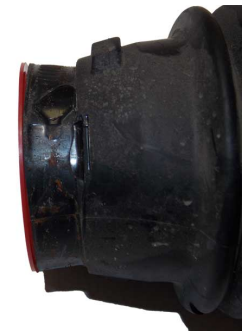
Figure 7: Red Plug Fully installed into firewall connector.
